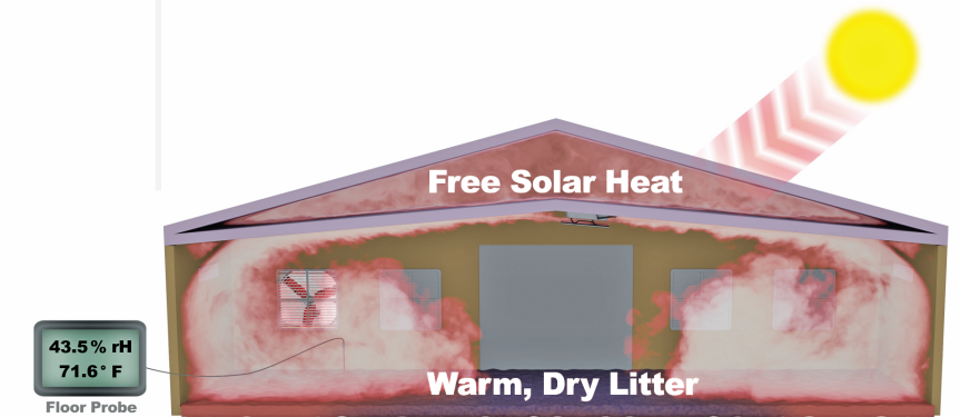
3D Rendering of attic inlet airflow in a poultry house
